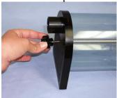
2) Remove the plastic lid from the flow chamber.
