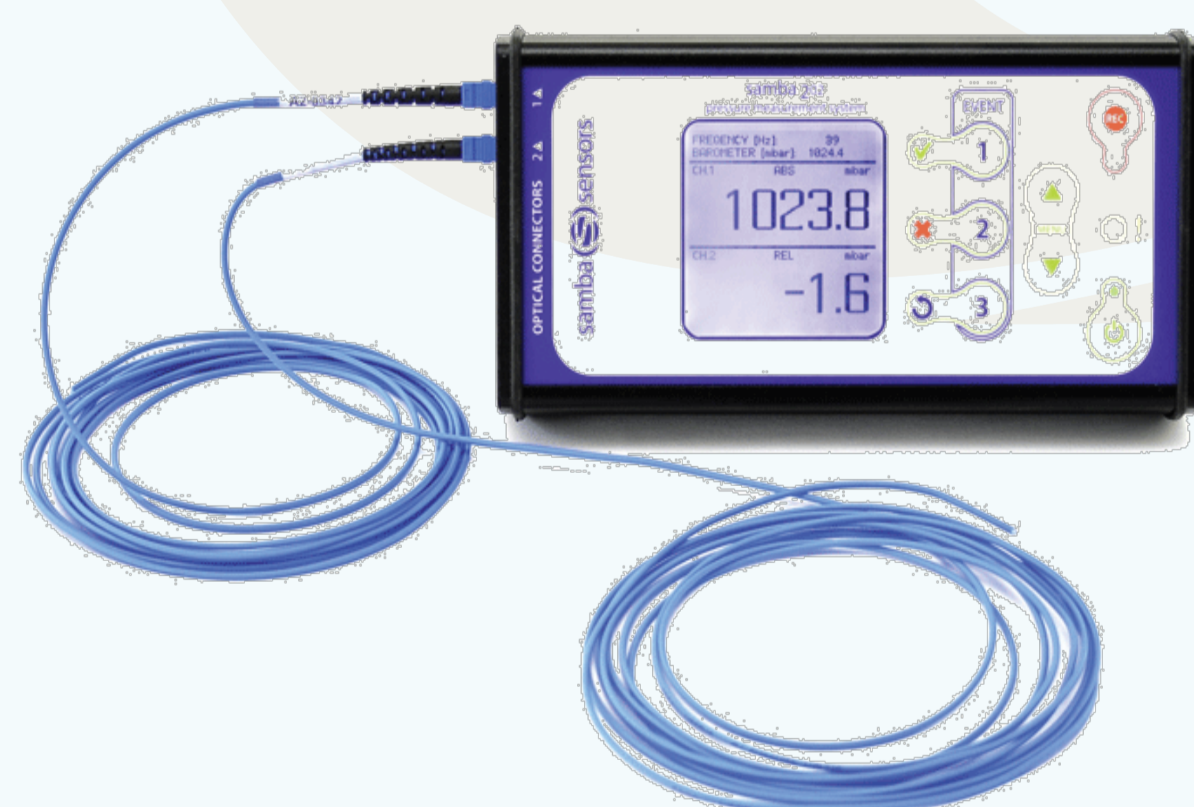
Figure 2. The Samba control unit.
