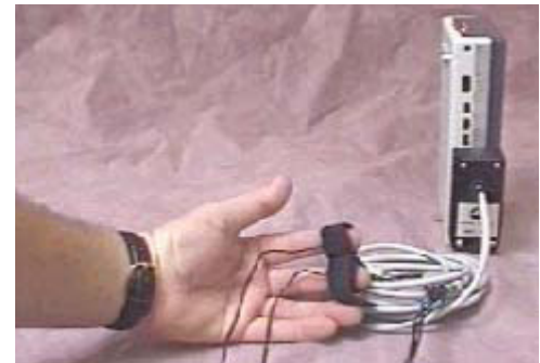
GSR100C shown with MEC100C and TSD203
