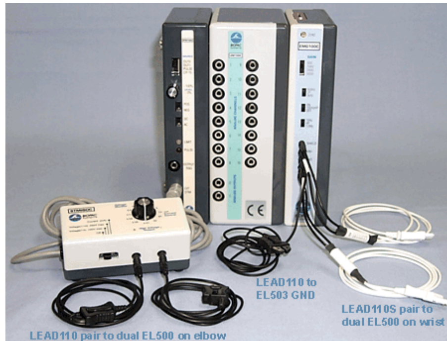
Figure 1: Amplifier setup and lead connections for recording nerve response
