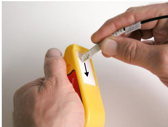
Figure 3 : Always clean the end of the connector ferrule before each connection
