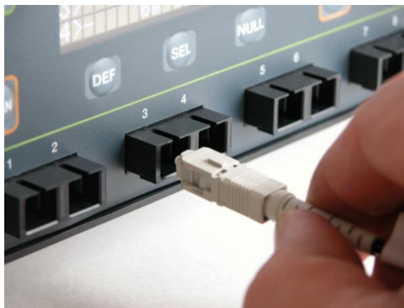
Figure 4 : Engage the sensor connector with the orientation key properly oriented and push until it clicks into place
