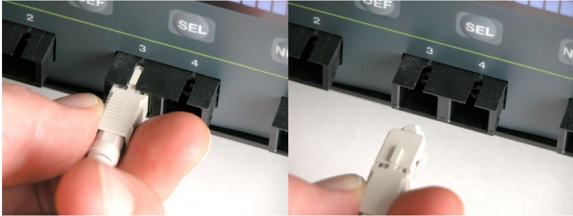
Figure 5 : To disconnect, grab the square connector body and just pull
