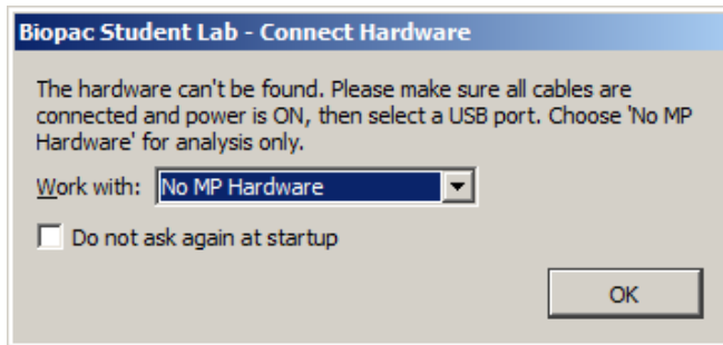
Fig. 6—Connect hardware prompt following BSL launch indicates possible failed driver installation
